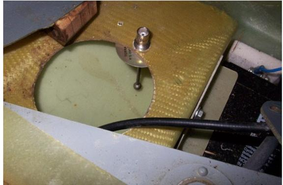
Ground plane removed from antenna
