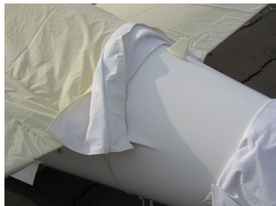
Blade antenna just behind wing
