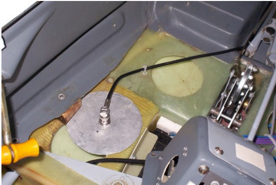
Rod antenna and ground plane mounted under thigh area
